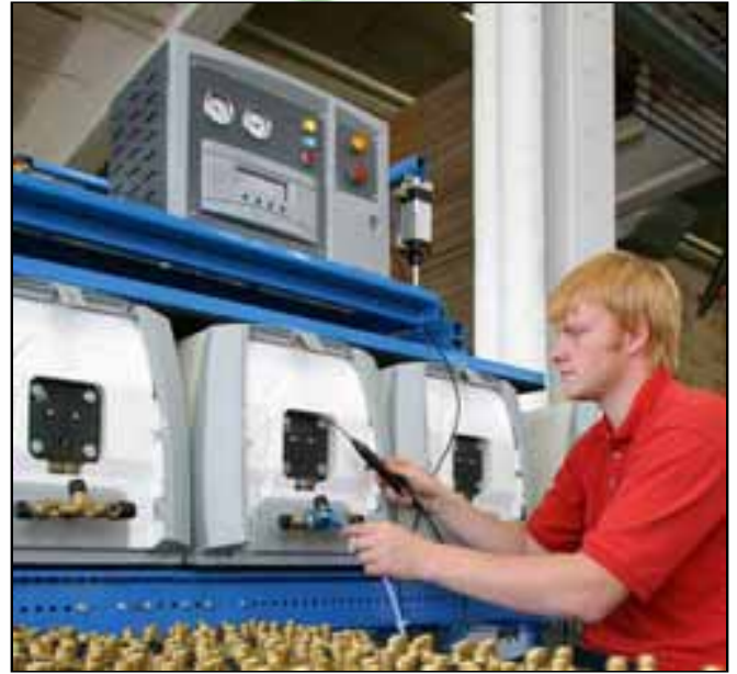
Leak Detection with Hydrogen Trace Gas
