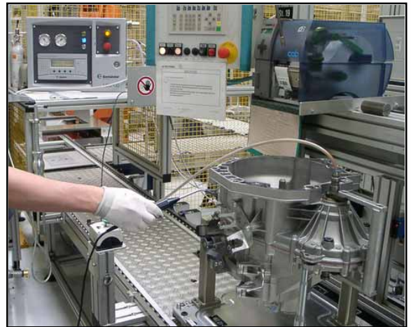
Fig. Leak Detection with Hydrogen Trace Gas
